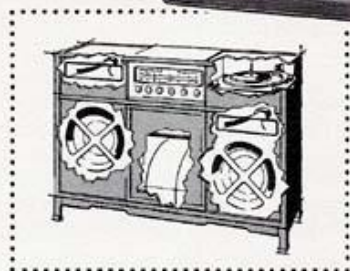
The cutaway illustration shows the two 15" bass speakers, two exponential horns, FM-AM-Stereo control panel and large record library compartment.
